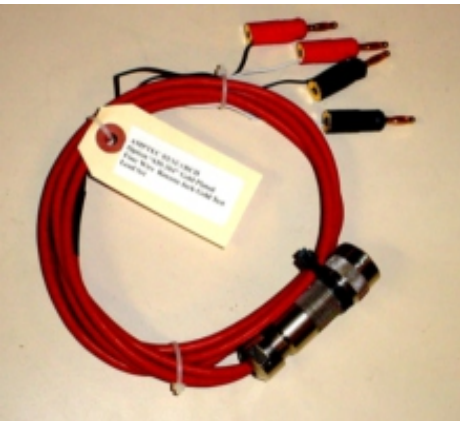
Option "630-304" Gold plated 4-Wire Kelvin Banana Jack Test Lead Set -
