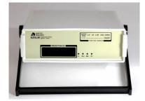
The AMPTEC 620LM Safety Igniter Tester is an ATE system dedicated portable digital ohmmeter specifically designed for ultra-safe resistance testing on squibs, igniters, flares, and other explosive devices. The 620LM provides ultrasafe measurements for THAAD related ordnance. With a built-in diode test capability, autorange, an RS232C Interface, and Optically Isolated Power, the 620LM will provide an effective measurement every time.
