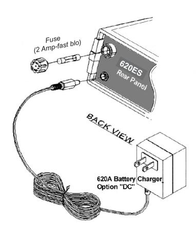
A fully charged battery pack typically powers the 620ES for approximately  $6 \sim 8$  hours before requiring a recharge. AMPTEC installs a quality set of 4 each Heavy Duty (5000 mAHr) Ni-Cad batteries. The 620ES will also operate on a 4000 mAhr  $\bf D$  cell Ni-Cads with a shortened operating time between charges. Recharge time is typically twice the "Power On" time. An "Overnight" charge usually restores the 620ES to a "Fully Charged" ready to use state.
