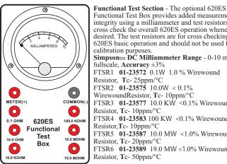
Functional Test Box provides added measurement integrity using a milliammeter and test resistors to cross check the overall 620ES operation whenever desired. The test resistors are for cross checking 620ES basic operation and should not be used for calibration purposes.
