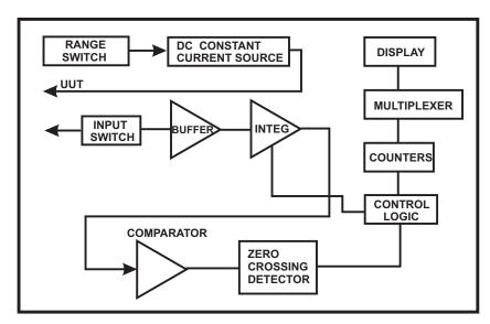
Figure E1 - AMPTEC 620ES FUNCTIONAL BLOCK DIAGRAM
