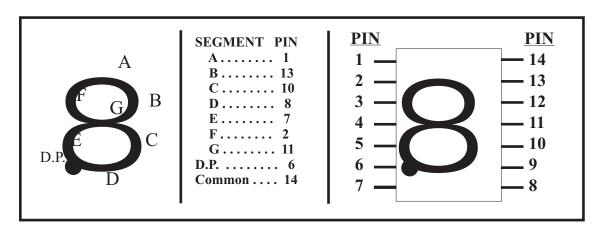
Figure E4 - 620 series LED Display Pin Out Detail/Functions
