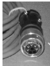
END VIEW TEST LEAD PLUG (remove dust cap from the bond meter) To plug in test leads, align and turn connector collar till you feel the “click”.
