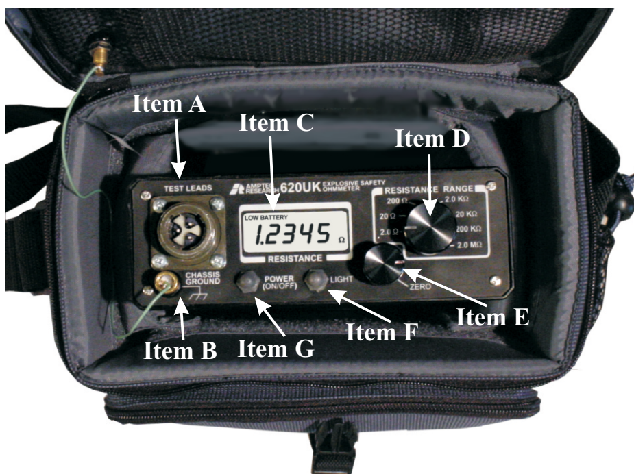
D-3 Photo of AMPTEC 620UK in Carry Case Earth Connection between Case and Ohmmeter is shown
